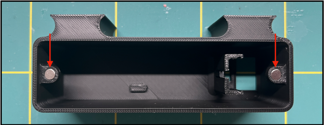
Figure 3: installation of the base magnets
