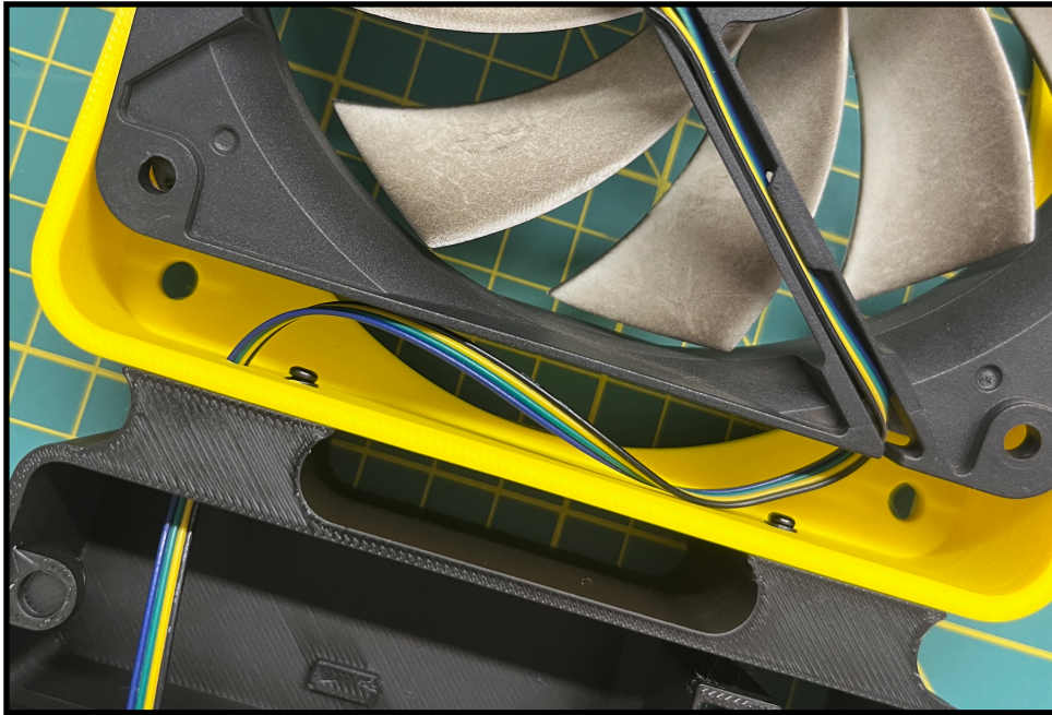
Figure 10: threading the cable
